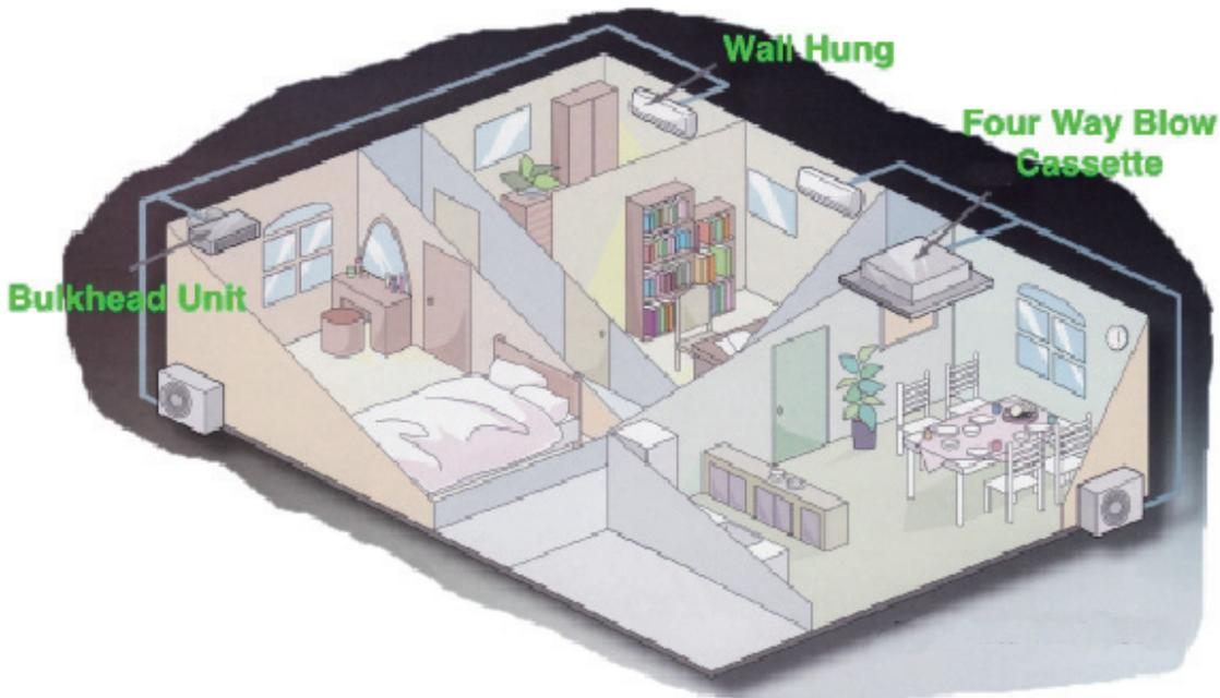
Figure 2: VRF Multi Split System (showing nine indoor units connected to one outdoor unit)
