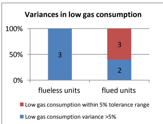
**Figure 3 Measured gas consumption rates against declared rates (low setting)**
