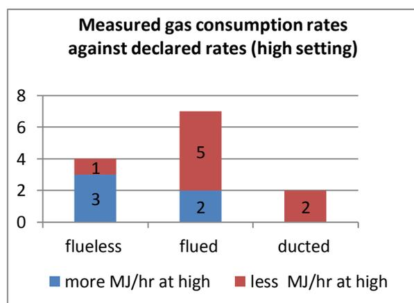
Considering that all flueless heaters consumed more gas than declared at low setting, and 2 out of 5 flued heaters were also not within tolerance, introducing a tolerance for this setting might improve the reliability of the energy label for these products.
