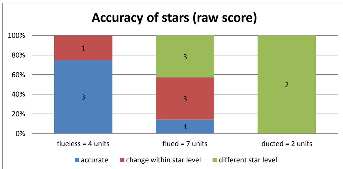
The tests results found that star ratings were inaccurately declared by 69% (9 of 13) of the tested gas space heaters.
