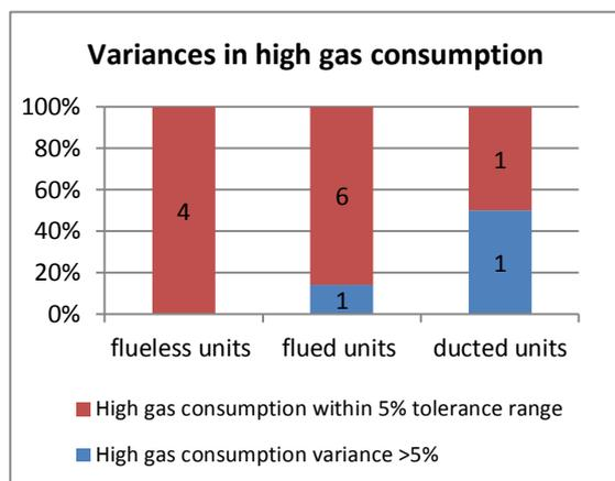
**Figure 5 Measured gas consumption rates against declared rates (high setting)**
