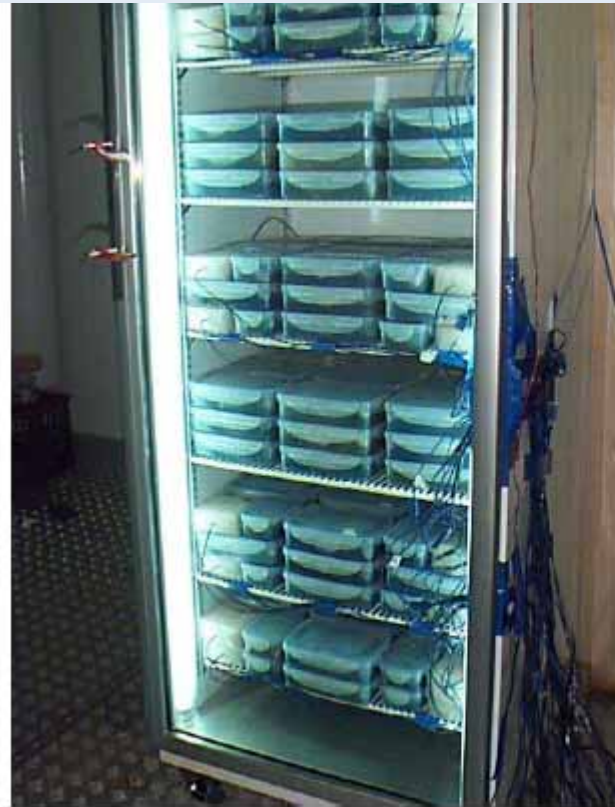
Figure 3.3 Mechlab Test Packs Loaded in Refrigerated Display Cabinet
