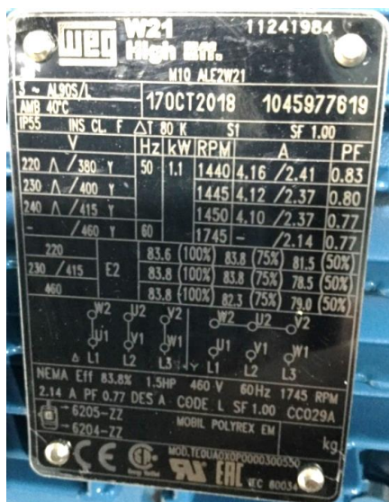
Figure 2: Rating plate – adequate details to confirm registration
