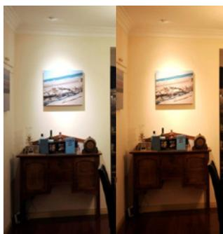
A cool white bulb is used on the left and warm white bulb on the right.
